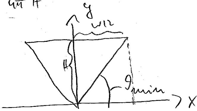
$$\omega I_{\min} = -\omega I_{\max} = \frac{w/2}{\sqrt{(w/2)^2 + H^2}}$$
