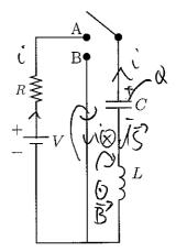
(b) At t=0 the switch is set into position B. Calculate the charge, Q(t), at the upper plate of the capacitor as a function of time!
