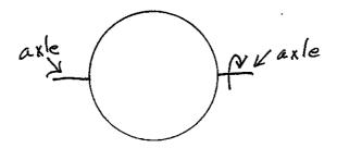
If a torque is applied to the axle, starting at t = 0, so that the loop has a constant angular acceleration,  $\alpha$ , find the current in the loop.
