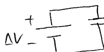
If we now connect the battery with electrically conducting wires, this potential difference will be applied to the capacitor.
