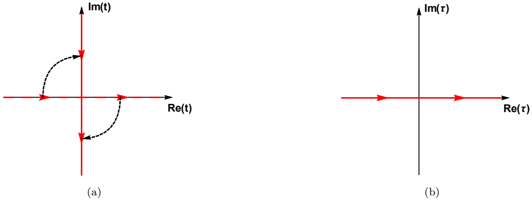
Figure 4.1: The diagram [(a)] shows the initial time-integration contour in Minkowski space-time (red dashed line), which is rotated clockwise into the complex time-plane (red line). The second diagram [(b)] shows the Euclidean time-integration contour, which corresponds to the Minkowski case of [(a)].
