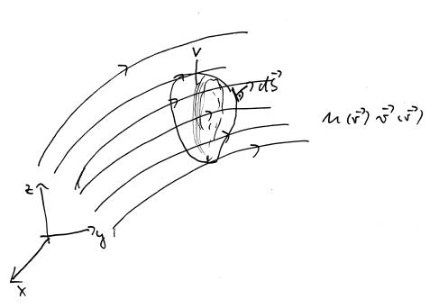
Flow of a fluid with particle density, n and velocity field  $\vec{v}$  through a volume, V.
