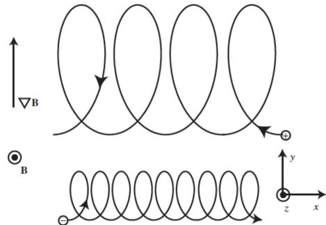
Consider r<sub>L</sub>=mv/qB, local gyroradius is large where B is small and is small where B is large which gives to a drift
