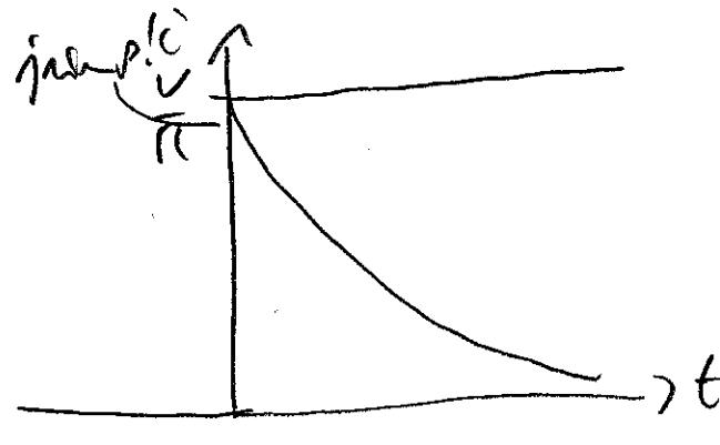
long-time limit: goes to steady state (i.e., no current and  $Q = CV$ , i.e., voltage of the capacitor becomes the voltage of battery).
