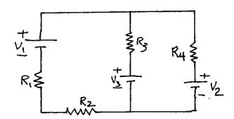
a. If no current flows through the resistor  $R_3$ , what current flows through  $R_2$ ? Call this current  $i_1$ .
